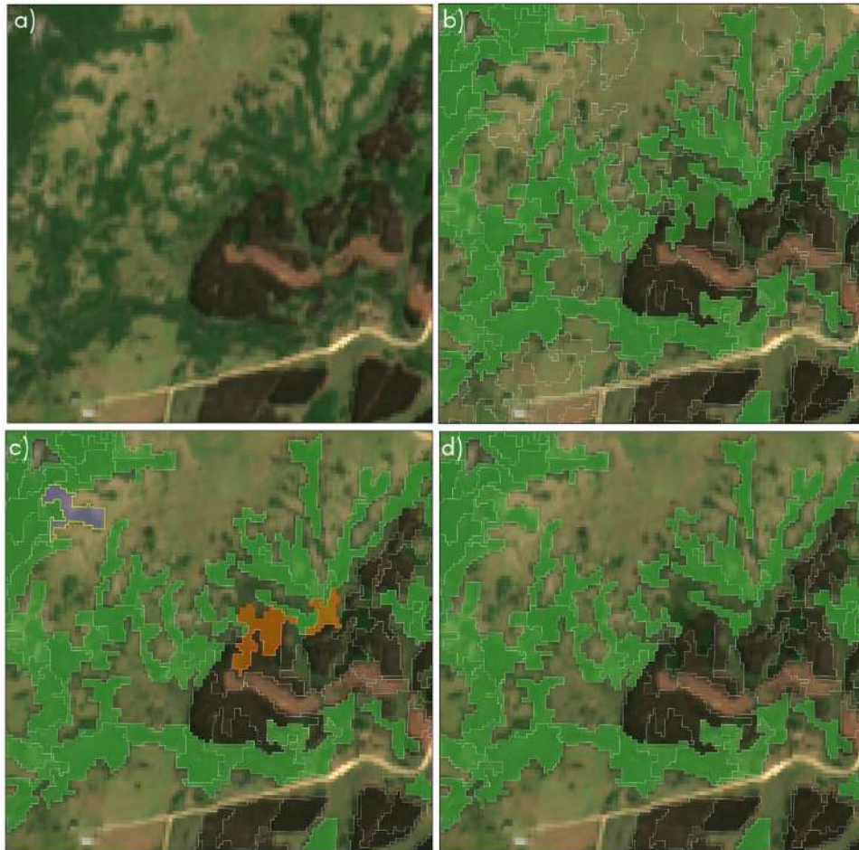
Figure 10: Example of the post-classification editing process: a) Sentinel-2 subscene in true color display; b) preliminary result of the native forest map (in green); c) preliminary result, highlighting misclassified segments, as Native Forest (in orange) and as Non-forest (in purple); d) post-editing result of the native forest map (in green).
